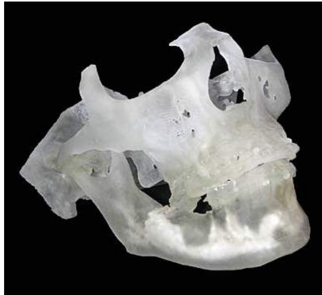
Figure C2: Physical prototype made using stereo lithography
